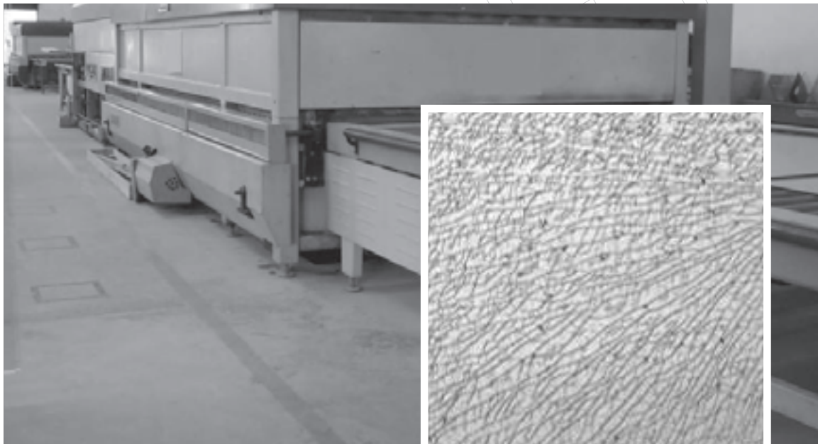
Tempered Glass - Breakage Pattern
